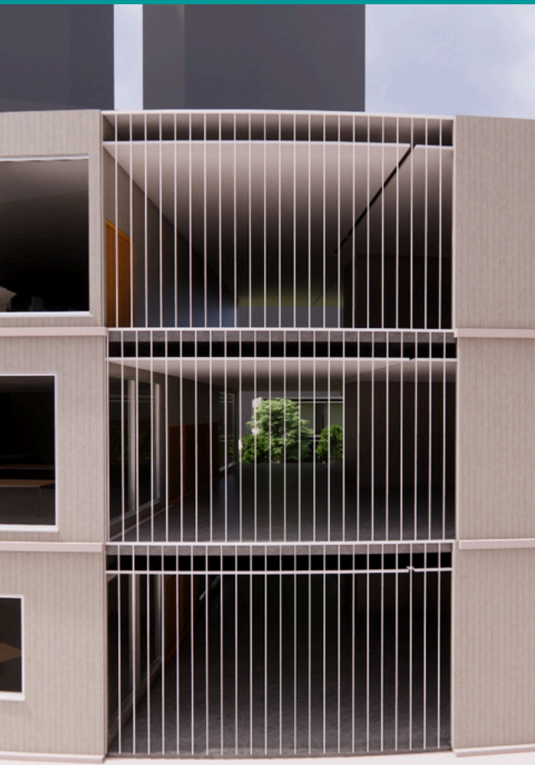
Exterior Perspective : Exterior louvres let wind pass through in.
