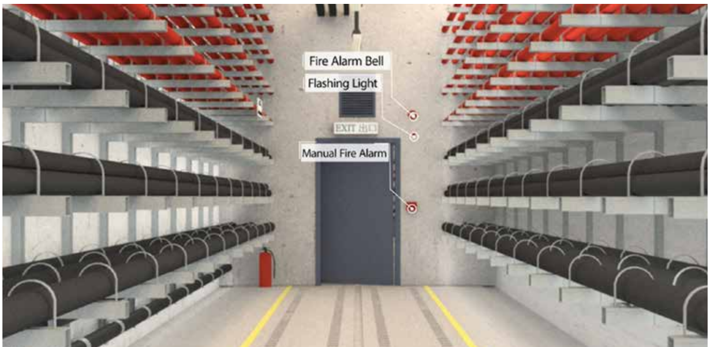
BIM Model provided an accurate sense of presence inside the tunnel that is yet to be built. Improvement to the design can be identified easily prior to the construction. Image courtesy of CLP Power Hong Kong Limited
