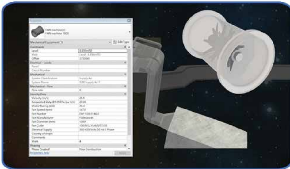
Accurate information of the building facility can be retrieved quickly in the BIM model for the facility management team. Image courtesy of CLP Power Hong Kong Limited
