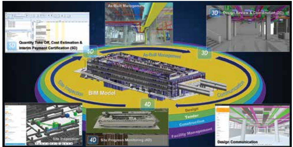
Full building life cycle approach with open BIM, open data concept from design to management. Image Courtesy of Urban Renewal Authority
