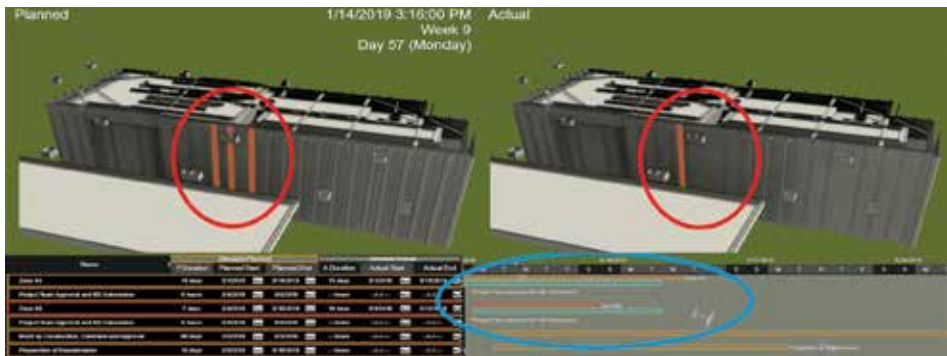
Phase planning 4D model adopted in the project for planning and construction programme monitoring. Image Courtesy of Urban Renewal Authority
